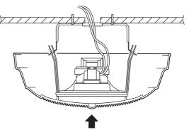
Push the speaker upward into position.
